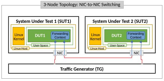
Server Systems Under Test (SUT) run DPDK Testpmd or L3fwd application in Linux user-mode as a Device Under Test (DUT). Server Traffic Generator (TG) runs T-Rex application. Physical connectivity between SUTs and TG is provided using different drivers and NIC models that need to be tested for performance (packet/bandwidth throughput and latency).
