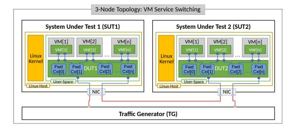
In "Chained" VM topologies, packets are switched by VPP DUT multiple times: twice for a single VM, three times for two VMs, N+1 times for N VMs. Hence the external throughput rates measured by TG and listed in this report must be multiplied by N+1 to represent the actual VPP DUT aggregate packet forwarding rate.
