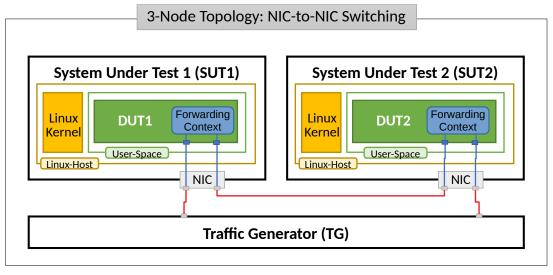
Server Systems Under Test (SUT) run VPP application in Linux user-mode as a Device Under Test (DUT). Server Traffic Generator (TG) runs T-Rex application. Physical connectivity between SUTs and TG is provided using different drivers and NIC models that need to be tested for performance (packet/bandwidth throughput and latency).
